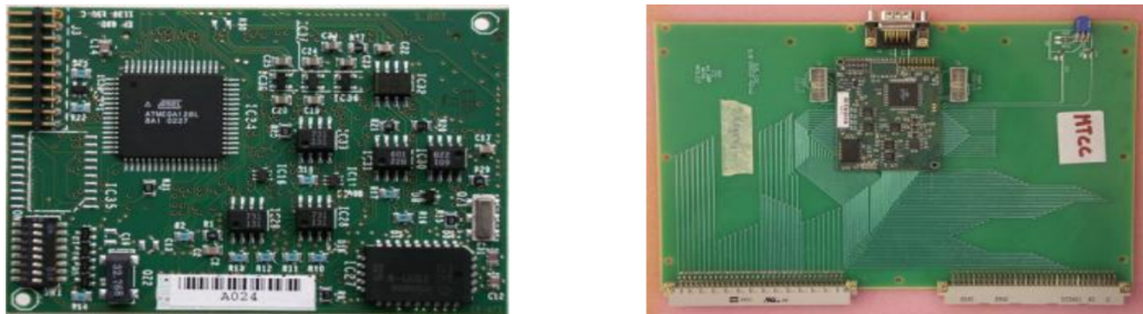
Figure 3.6: Photographs of ELMB and custom made PTM/HM electronic boards [31].
